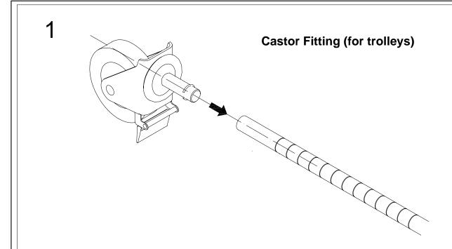
Press caster stems into bottoms of posts until fully engaged. Use a rubber mallet or hammer wrapped in a towel to tap casters firmly in place.
